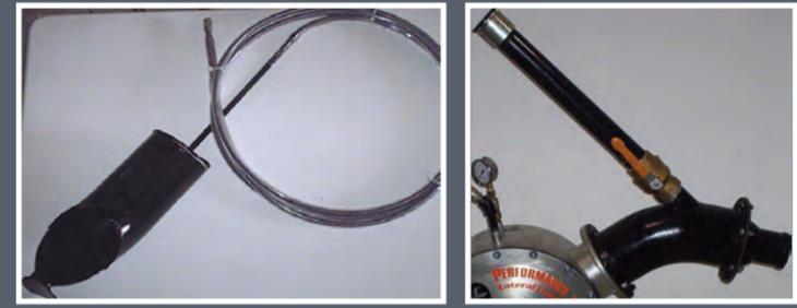
The process includes the use of a camera port which allows a lateral push camera to be inserted inside the translucent bladder, providing visual verification of the liner placement prior to curing.
