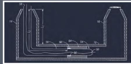
The liner can virtually begin anywhere in a pipe and applications are not limited to lateral pipes. Another application for this new technology occurs when a mainline pipe has only one manhole access.
