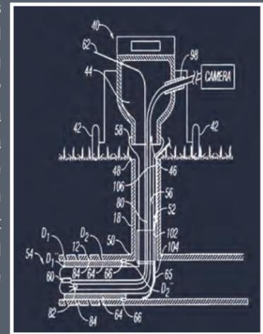
Another aspect of this new technology includes the use of a camera port. The camera port is a pressurized port where a lateral push camera is inserted in the interior of the translucent bladder. The camera provides visual verification of the liner placement ensuring that the liner started in the proper location and that the liner is fully inverted, not protruding into the municipal main pipe.
